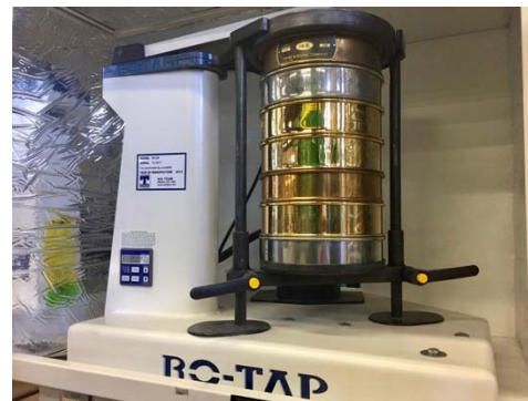
Figure 1: Image of the Ro-Tap sieving system used in the laboratory analysis of kernel processing.
