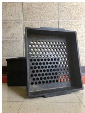
Figure 2: Image of the Penn State Particle Separator for determination of particle distribution in silage samples.
